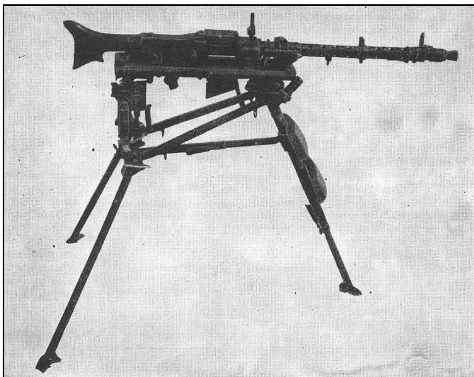
M.G. 34, caliber 7.92 mm, on tripod mount as heavy machine gun.
