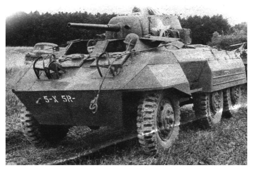
ARMORED CAR, M8, 6x6, the Army's latest combat vehicle, is a six-wheeled, eight-ton armored job that can hit high speed over practically any type of terrain. It mounts a 37-mm cannon and a .30-caliber machine gun in a hand-operated traversable turret. The M8 carries a crew of four and is intended primarily for use in reconnaissance combat.
