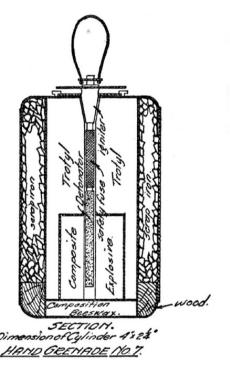
Hand Grenades Nos. 6 and 7 consist of metal cases filled with T.N.T and a composite explosive and are exactly alike, except that No. 7 contains shrapnel bullets or scrap iron, while No. 6 contains only explosive. At the top of each case is a place to fix the friction igniter, which is supplied separately. When these bombs are to be used, detonator fuse and igniter are put in and firmly fixed. Before throwing the becket on, head of igniter should be pulled smartly off.
