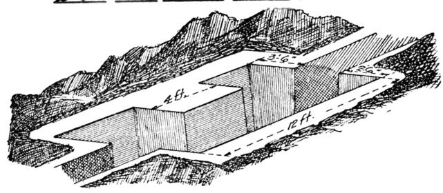
Dimensions variable. Note the wide berms permitting the use of strong roof supports. A layer of large stones to cause early shell burst should form part of the roofing.
