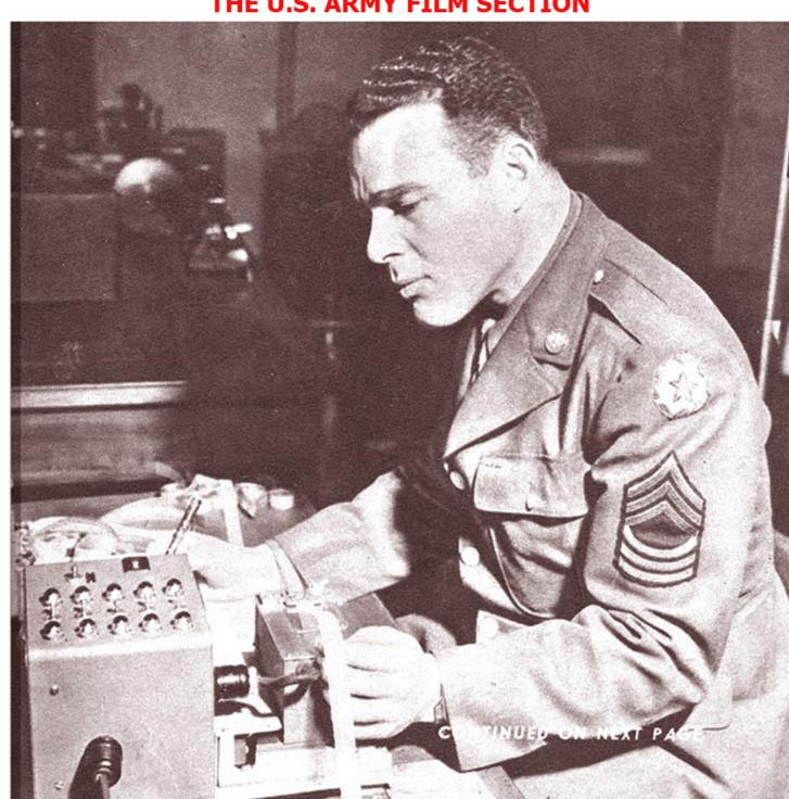
WHEN REVIEWER throws a switch, perforations are made on paper tape synchronized with movie film. This sergeant checks individual requests.
