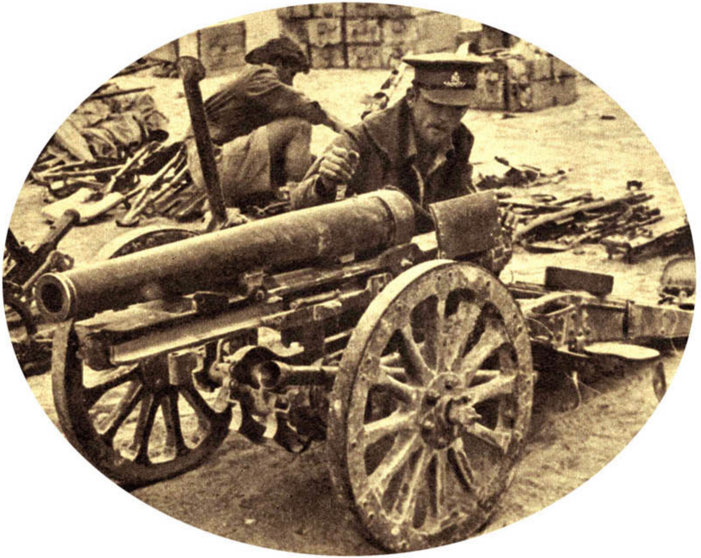
BRITISH OFFICER CAREFULLY CHECKS BREECH OF AN ARTILLERY PIECE ON BATTLEFIELD. HIS ANALYSIS REPORT WILL ACCOMPANY GUN BACK TO AN ALLIED ORDNANCE CENTER
