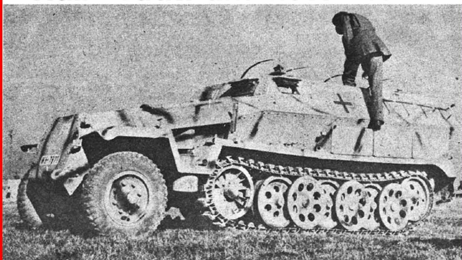
The German armored half-track personnel carrier is a six-cylinder, 100-horsepower job with a maximum speed of 40 mph. It carries two MG34 machine guns. This vehicle has a coffin-shaped body, and carries 10 men on two longitudinal seats. One machine gun is mounted to the right of the driver, whose visibility is limited to two small glassed-in slots as shown above.
